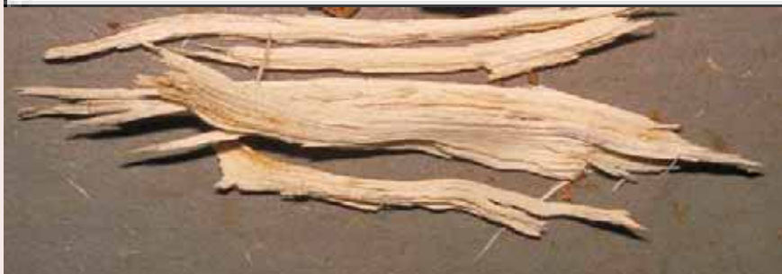
White rot in aspen (left) and brown rot in oak (right)
