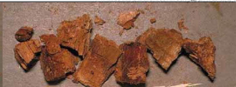
White rot in aspen (left) and brown rot in oak (right)
